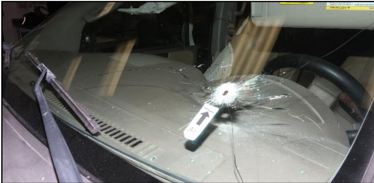
Above: Defect in the driver's side front windshield of the Nissan Armada.
